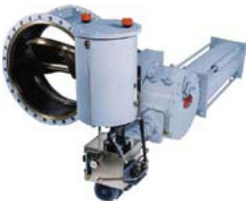
Triple-offset metal-seated rotary process valves with quick-closing hydraulic actuation package for the turbine trip valve, and a modulating hydraulic actuation package for the turbine throttle valve.
