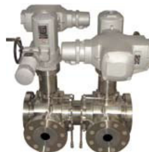
Tandem metal seated ball valves with emission leak test ports and electric motor operated. The actuation can be set-up with sequential operation lock-out.
