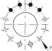
\* Knife-gate valves 3" will be delivered in 8-hole flange execution!
