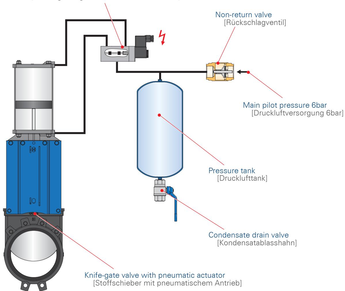
Knife-gate valve with pneumatic actuator
