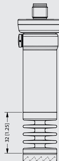
P42 | High-temperature version with cooling section
