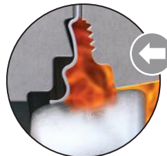
Line pressure applied from non-preferred flow direction. (During or after fire event.)
